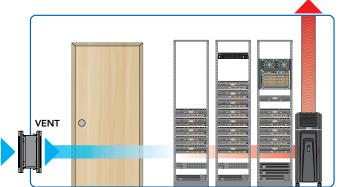
SRCLOSETINTAKE for inflow combined with a portable cooling unit like the SRCOOL12K that vents warm air via its duct.
