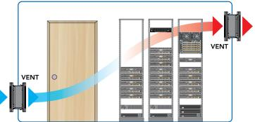
Passive cooling solution combining (2) SRCLOSETINTAKE vents, positioned to take in cool air and expel warm air.
