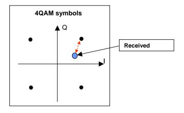
The switchover between two adjacent ACM profiles is triggered by the crossing of an upper or lower MSE threshold for each modulation level.
