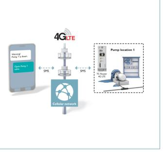
Monitor and control a remote water pump via SMS.
