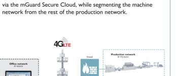
Use a TC mGuard RS4000 to access a remote machine network
