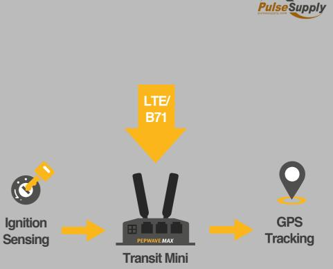
The MAX Transit Mini provides cellular connectivity for passengers. It connects using LTE, supporting band 71 for improved range and signal penetration. This means the Transit Mini will stay connected even in remote areas where other bands drop off.
