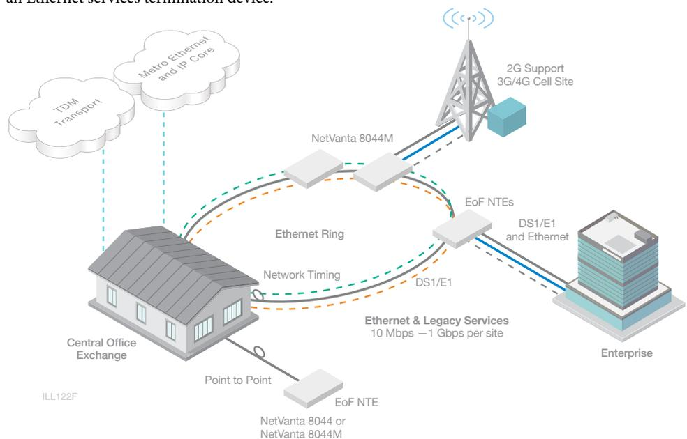
**The NetVanta 8044M supports two variations of fiber access topology: Point-to-Point and Ethernet ring to deliver both legacy ATM/TDM and next-generation IP/Ethernet services.**
