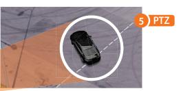
The Advanced PTZ Handover is a quick and simple to program function that triggers camera presets and automatic target tracking based on detected events.
