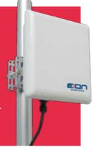
Use of intelligent antenna systems and advanced WiMAX features is what allows the StarMAX SS to offer market-leading performance. The variants available, the StarMAX 2120, 2160 cover indoor, and outdoor deployments respectively.
